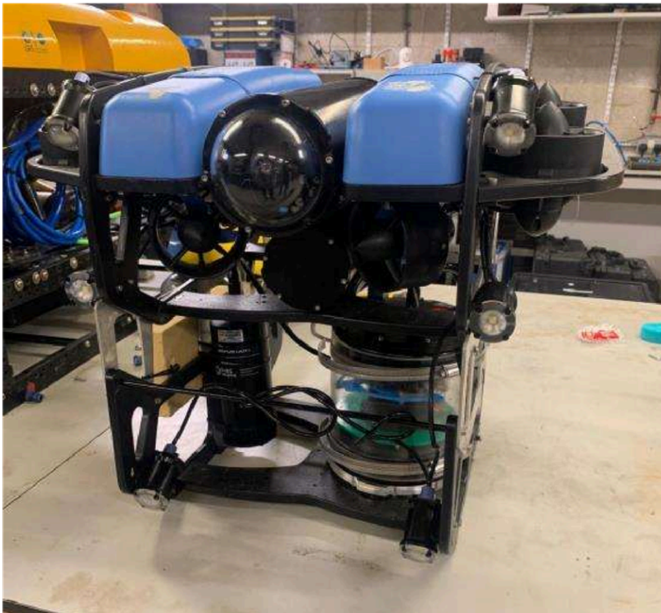
Figure 1: BlueROV system modified with the custom camera and lighting configuration used for autonomous reef data acquisition.
